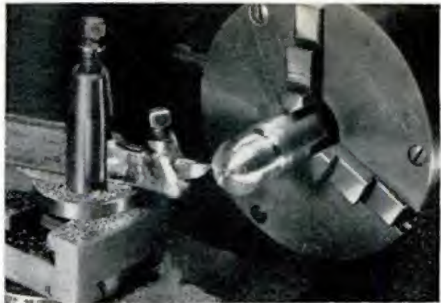
THE 1-IN. BALL is first roughed out with conventional tooling to save wear and tear on ball turner
